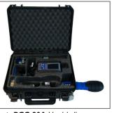
▲ PCC-20A Hardshell case holds AdvancedSense BE, probes (DSII internally, or extended during secure monitoring) & accessories.
